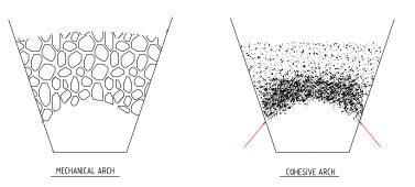
It is easy to tell if a silo has a material flow problem by looking for 'hammer rash' on the wall. If the product is not moving freely through the silo and outlet the operator will strike the side walls to rattle the material free.
